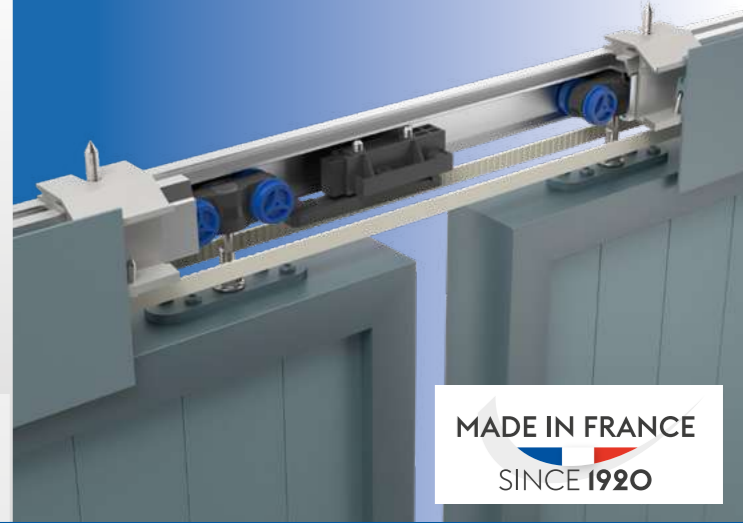
Ceiling mounting - single channel - 2 synchronised symmetrical leaves
